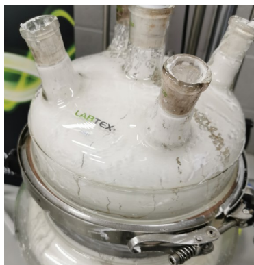
Figure 2: calcium carbonate accumulation on the feed vessel lid
