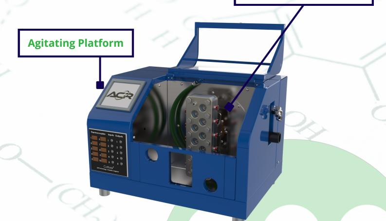
The **Agitating Platform** provides lateral motion to the reactor block, generating mechanical mixing.
