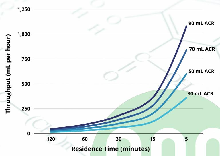
In any flow process, **productivity is directly linked to the reaction residence time.** A shorter residence time allows for greater productivity from a single system.
