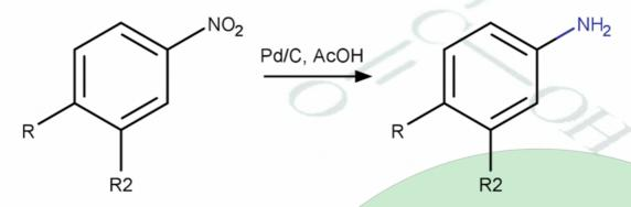
Hydrogenation of an aromatic nitro compound to yield the corresponding amino compound has been performed at pressures under 10 bar and with rates of conversion **twice as fast** as equivalent batch processes reported in the literature.
